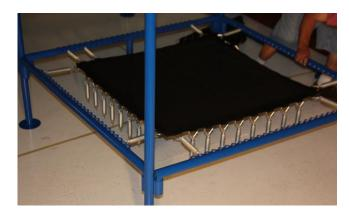
Tip! If the springs are too stiff to stretch by hand, use the spring tool provided (part #99)
