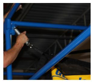
Attach the housing to the loops. Use the spring tool to stretch the springs if needed. Start with from top and move down. Repeat for the other housing.
