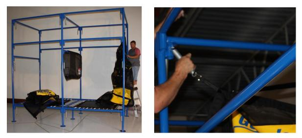
Use the spring tool to stretch the springs if needed. Start with from top and move down. Repeat for the other 3 housings. Ensure that #63L and #63R are on opposing corners.
